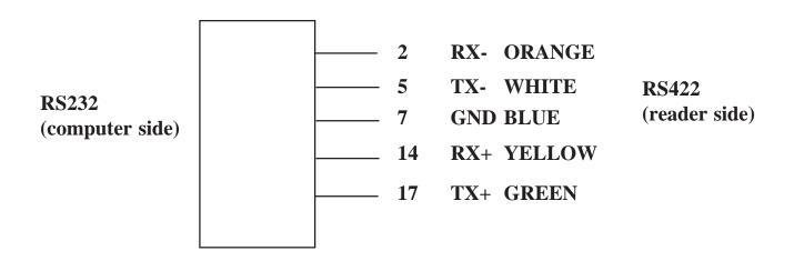
Note: If you make a cable for the RS232 side, make sure that pins 7 and 8 are connected to each other (shunted).
