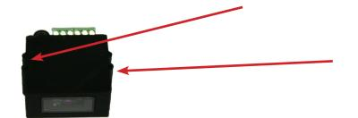
Qscan Mini is mounted using 2 #4 screws at these locations.
