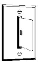
Mounting the reader is performed just like mounting a wall plate, with two screws that screw into a standard gang box.
