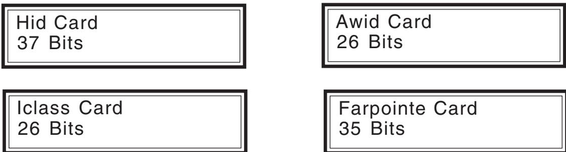
Press the button on the side of the Proxcheck. This moves you to the next menu. On the next menu, Proxcheck will display a binary bit dump of the card. The first screen will display bits 1 through 16. Pressing the button again will display additional bits, 16 at a time, until all the bits on the card have been displayed:
